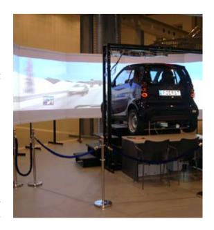
generates original sounds according to the situation (starter, engine noise, horn, screeching of tires, drive wind, rain, etc.) and the driver's sight system includes five large screens surrounding the Smart cabin driving simulator.
